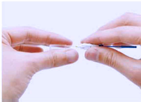
05. Take the fiber protector off from the ferrule.
