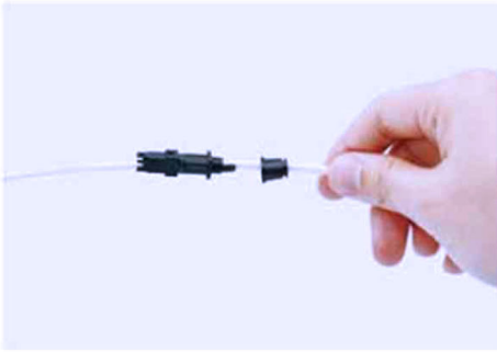
01. Pass the cable through the boot and the boot cap.
