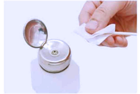
03. Clean the stripped cable with alcohol soaked tissue.
