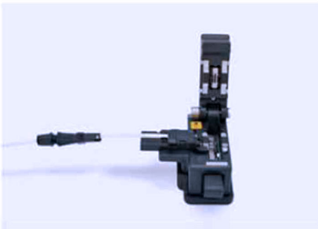
04. Cleave it with a cleaver.
