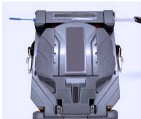
08. Put the spliced connector in the oven, then it will start heating automatically.
