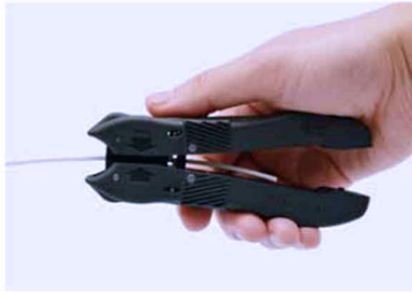
02. Strip the indoor cable with a stripper.
