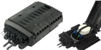
The Snap Lock Combi Closure is an enclosure with key design features, ease of operation and a high degree of ingress protection. There is one uncut cable port (for cable diameter D10°D17.5mm), 16 small cable ports (cable diameter less than 4mm), 2 branching-cable ports (cable diameter D8°D17.5mm by changing sealing units).
