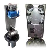
A traditional dome enclosure featuring a unique internal structure, designed for an adapterconnector solution as an alternative to the fusion splicing system. This unique closure features a strong and secure metal internal plate with a fibre management system in the rear
