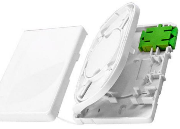
Dimensions (including lid) Length: 124.24mm; Width: 79.2mm; Height: 26.1mm OPTiFab's 4 fibre FTTx box is constructed from a lightweight & strong ABS material. It features a compact design with a sliding removable cover for ease of access during installation. It features front and rear cable entry points for 3mm or 5mm cable.
