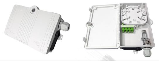
The 4-way lock and latch wall box is used for the distribution & termination of fibre optic cable devices. The IP65-rated wall box can be utilised for FTTH applications & other installation requirements to break out and splice input cables into drop cables, pigtails or direct patching. The box may also be used for protective interconnection of a fibre network and is suitable for outdoor, riser and tunnel installations.
